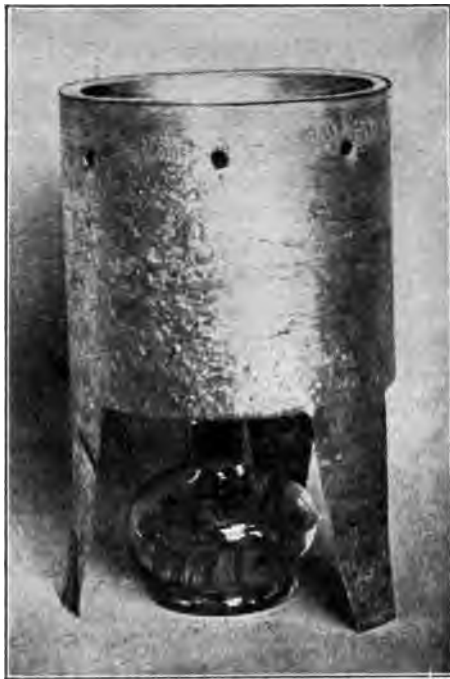
FIG. 32.—A simple apparatus for fumigation, from piece of stove pipe.
